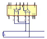
Network termination- Place  $120\Omega$  termination resistor at each end of the network
