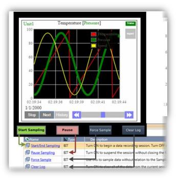
When the remote viewer accesses Live Trends via, the viewer can click Inspect to display sampling points and hover a cursor over a point to view its value.
