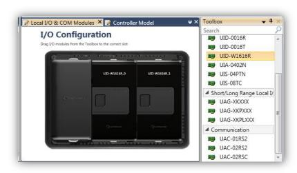
New Temperature I/O Module UIS-08TC is a standard-sized Uni-I/O™ module.
