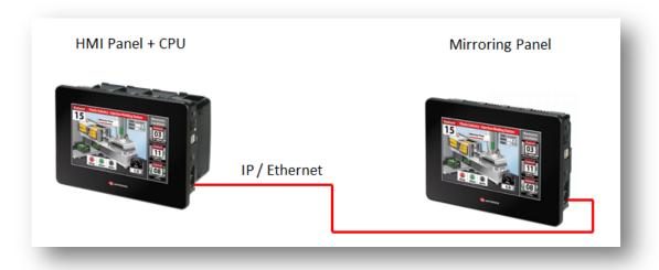
Simply open VNC Client on the 'mirroring' panel and enter the connection settings of a remote panel + CPU. Next, under CPU Control, select Ignore CPU events.
