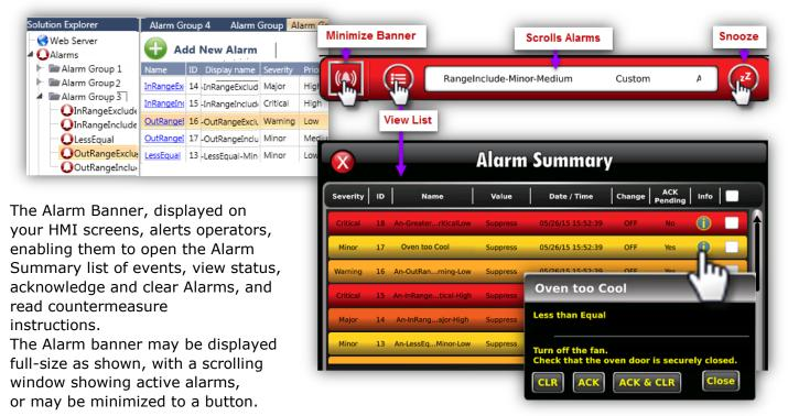
The HMI Toolbox now includes a new widget: the Alarm Status Viewer. This allows convenient Alarms management.
