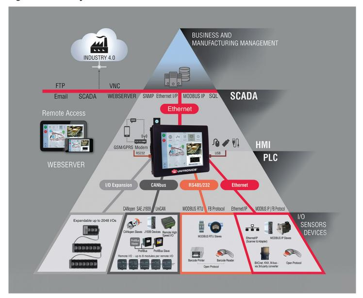
The unique features of Unitronics All-in-One PLC + HMI controllers enable them to play a central role in production factory and manufacturing enterprises.
