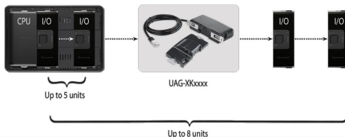
If a UAG-XKxxxx follows another adapter with an integrated power supply, the support capacity of that powered module limits the number of Uni-I/Os that can be connected to the UAG-XKxxxx; in any event, no more than 8 Uni-I/Os can follow a UAG-XKxxxx adapter.
