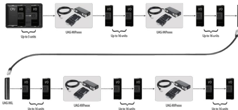
Configurations with Short-range adapter, no Power Supply (UAG-XKxxxx).
