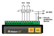
Shields should be connected at the signals' source.
