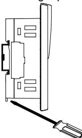
**Note:** Removing the unit requires clearance space. Recommendation: approximately 40mm (1.58”).
