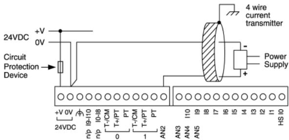
Analog Input wiring, voltage, AN4 and AN5
