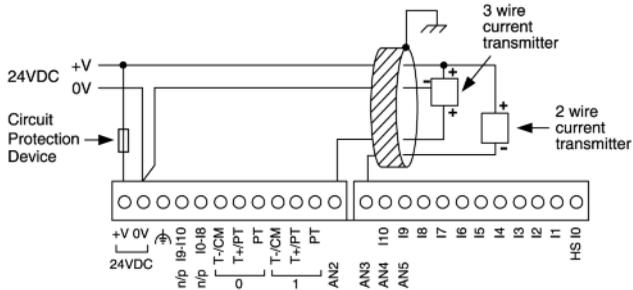
Analog Input wiring, current, 4 wire, AN2 and AN3
