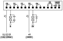
Transistor pnp output wiring
