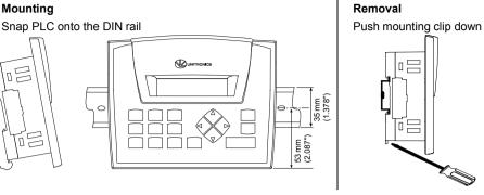
Note: Removing the unit requires clearance space. Recommendation: approximately 40mm (1.58").
