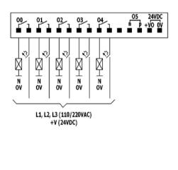
Transistor npn output wiring
