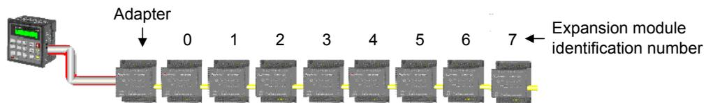
The formula below is used to assign addresses for I/O modules used in conjunction with the M90 OPLC. X is the number representing a specific module's location (0-7). Y is the number of the input or output on that specific module (0-15).
